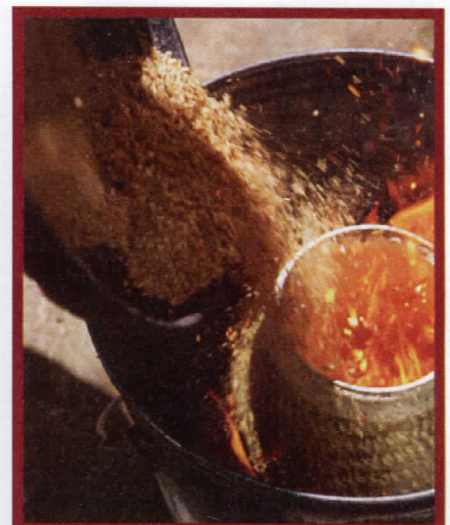
After sufficient spraying, the piece is placed in a small metal container, sprinkled with coarse sawdust, allowed to flame, then covered.
