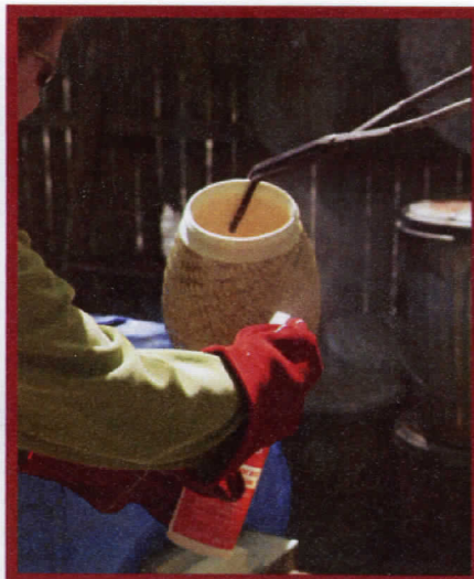
Next, he sprays areas of the surface with water. This brightens the glazes and reduces the likelihood of copper lusters. You can also control cooling by pouring water onto your piece as you would pour a glaze, or by using compressed air.
