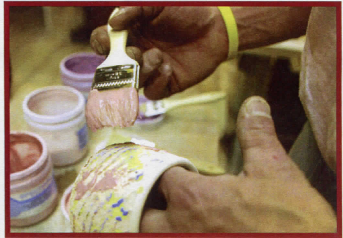
I apply multiple thin layers of glaze by drawing the brush lightly over the surface of the pot.
