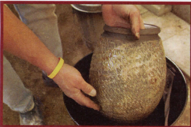
Being patient and allowing the piece to cool to the touch before opening the container all but eliminates cracking due to fast cooling.
