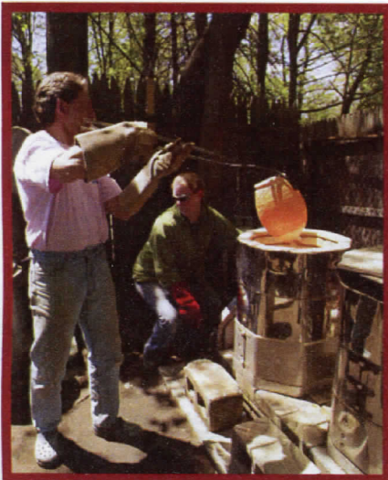
In this photograph, my assistant has just removed the lid so I can retrieve a larger piece with tongs.
